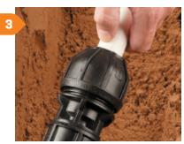
Insert the pipe to the correct depth. Always ensure the nut is backed off and 3 threads are showing. Pipes at the topend of the fitting tolerance may require 5 threads showing.
