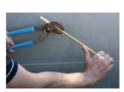
5. Using a pair of multi-grips or equivalent the lever can then bebent to the necessary angle.
